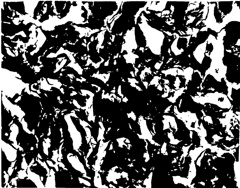
Fig.54. TEM micrograph of MX-80 clay matured at room temperature, acrylate-treated and ultramicrotome-cut. Magnification 13 000 x
